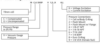
For example: Part #19C100PV4K = 19 mm Cell, Comp., 100 psi, Vacuum Gauge, 1/8NPT Port with 10 Vdc excitation.
