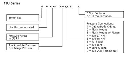
For example: Part #19U100PA4K = 19 mm Cell, Uncompensated, 100 psi, Absolute, 1/8NPT Port with 5 Vdc excitation.
